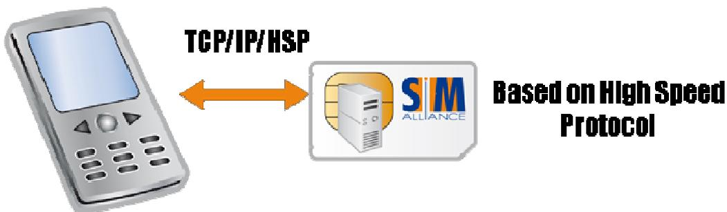
The SCWS can be used with BIP (Bearer Independent Protocol) over the ISO 7816 interface or with a full TCP/IP stack over the New UICC-Terminal interface USB.
