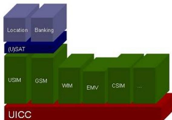
With the deployment of always-on LTE networks, the UICC is transformed into an IP-connected multi-application platform, allowing consumers to securely access a host of IP- and cloud-based services and applications - from banking through to presence-based instant messaging. But more than this, with storage now in excess of 2 GB, the card is also a secure applications store for a host of services
